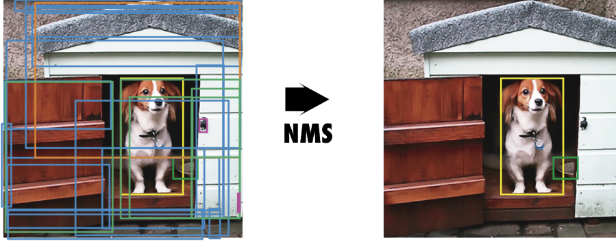
Figure 3: Non-Maximum Suppression (NMS). a) Shows the typical output of an object detection model containing multiple overlapping boxes. b) Shows the output after NMS.
