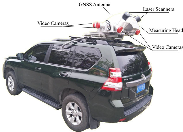
Fig. 2. Acquisition system consists of two laser scanners, up to six video cameras, and a combined IMU/GNSS system.
