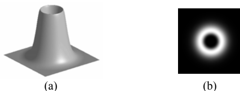
Fig. 1: An example of the log-Gabor filter in the frequency domain, with \omega_0 = 1/6 and \sigma_F = 0.3 , shown in 3D surface format (a) and in gray-scale image format (b).
