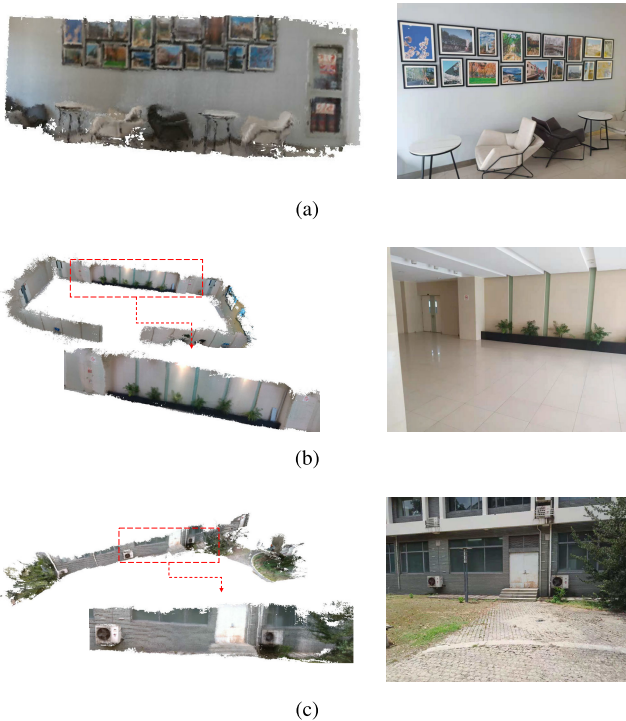
Fig. 5. Typical samples of reconstructed dense maps. From (a) to (c), the results correspond to the single-agent indoor mapping, the multi-agent indoor mapping and the multi-agent outdoor mapping, respectively. And in each group, the yielded dense map of CVIDS is shown on the left, while the snapshot of the real scene is on the right.
