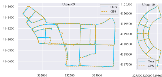
Fig. 8. Localization results of D-LIOM in complex urban environments. Despite the fact that GPS is not very reliable under the shelter of towering structures, the trajectories aligned with GPS show that our D-LIOM can nevertheless produce globally consistent localization results when running for a long time in large-scale scenes.
