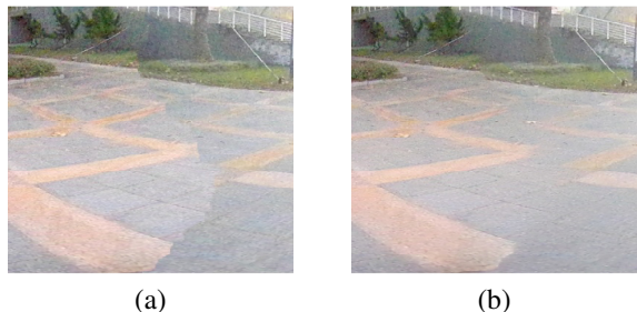
Fig. 4. The effect of multi-band blending. (a) is a fused image without multi-band blending and (b) is (a)'s counterpart with multi-band blending.
