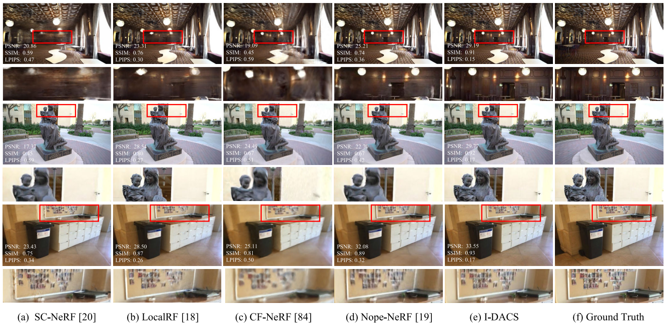
Fig. 4. Typical samples of the novel-view synthesis results of compared methods. In each group of data, the full synthesized views are shown on the top and the enlarged local ROIs are on the bottom. The results of the top two scenes are from the tanks and temples dataset [81], and the bottom one is from the Scannet dataset [80].
