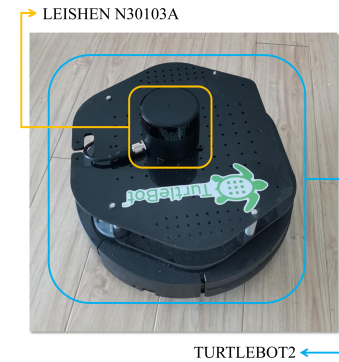
Fig. 5. Real-world experimental platform. Our experimental platform is composed of a TURTLEBOT2 robot platform and a LEISHEN N30103A single-line LiDAR with 360° viewing angle and 30m measuring range.
