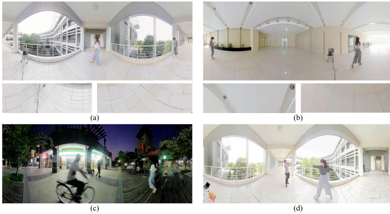
Fig. 13. Failure cases. (a, b) Failure cases caused by cylindrical projection. (c) A failure case of seam-cutting caused by motion blur. (d) A failure case of photometric alignment.
