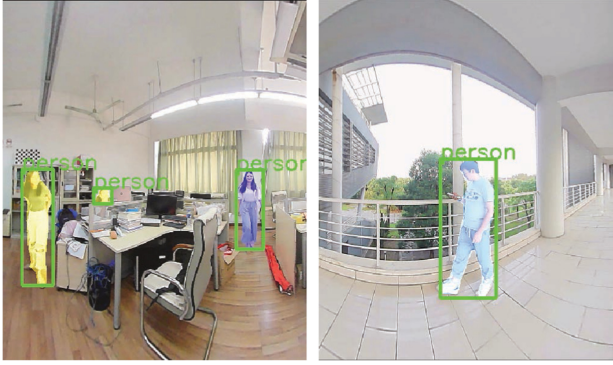
Fig. 7. The segmentation result of the person category by Mask R-CNN [14].
