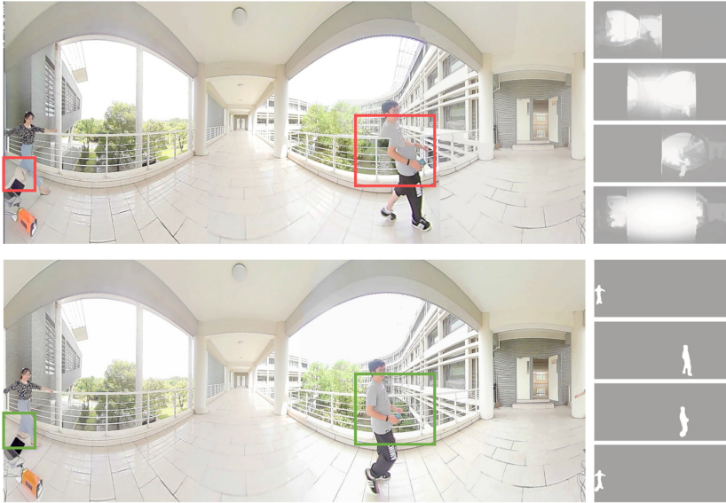
Fig. 1. Comparison of different seam-cutting algorithms. The upper images are the result of a visual saliency-based scheme [29] and corresponding visual saliency maps of images to be stitched. The visual saliency strategy failed in such a panorama scene, and the seam cannot avoid the pedestrians. The bottom images are the result of our instance segmentation-based scheme, which can accurately segment the pedestrians and ensure their integrity.
